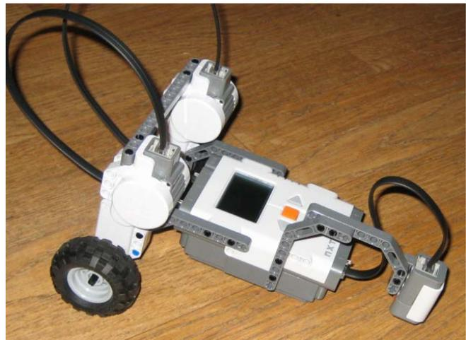
*Example of a simple line-following robot*
