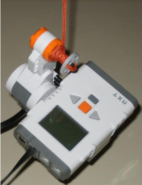
*Example of a simple rope-climbing robot, which reels in the rope*
